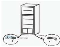
Unscrew and remove the bottom right hinge. Reserve the screws. Remove screw covers from opposite corner (left) and cover exposed holes (right). Attach bottom left hinge with the reserved screws.
