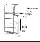
Unscrew and remove the middle hinge and middle hinge washer. Reserve the screws. Lift the refrigerator door up and away from the appliance.
