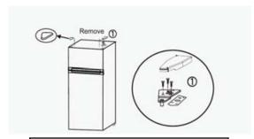
Remove top hinge cover. Unscrew and remove the top hinge and top hinge washer. Reserve the screws.
